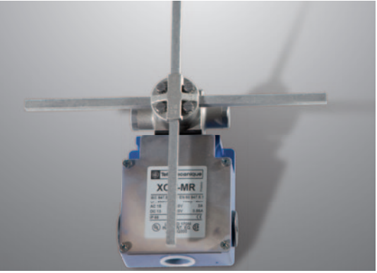
Travel limit switches for cross and long travel. Pre-switching and limit switching in both directions of travel.
