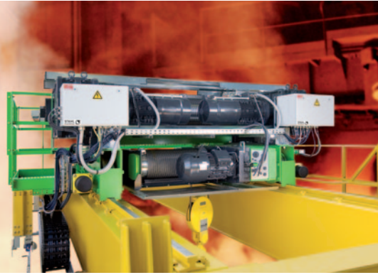
As standard with two synchronously controlled hoists and brakes.
